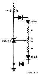
FIGURE 2. Temperature Coefficient Adjustment (Trim Range = ±0.5V Typical)
