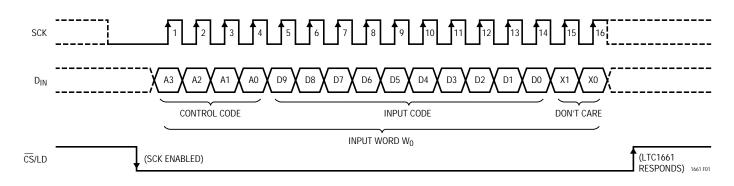
Figure 1. Register Loading Sequence
