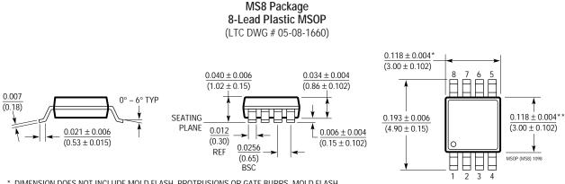
\* DIMENSION DOES NOT INCLUDE MOLD FLASH, PROTRUSIONS OR GATE BURRS. MOLD FLASH, PROTRUSIONS OR GATE BURRS SHALL NOT EXCEED 0.006" (0.152mm) PER SIDE
