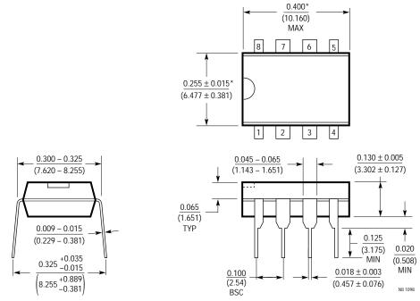
\*THESE DIMENSIONS DO NOT INCLUDE MOLD FLASH OR PROTRUSIONS. MOLD FLASH OR PROTRUSIONS SHALL NOT EXCEED 0.010 INCH (0.254mm)
