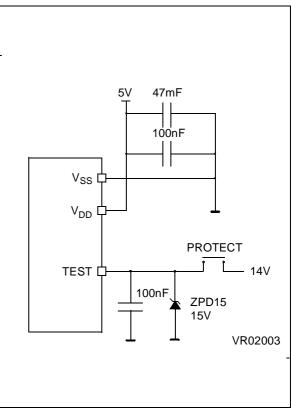
Note: ZPD15 is used for overvoltage protection
