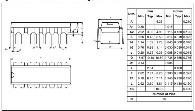
Figure 46. 16-Pin Ceramic Side-Brazed Dual In-Line Package
