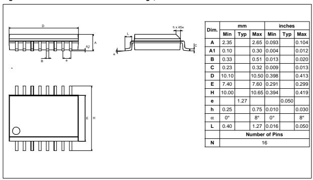
Figure 48. 16-Pin Plastic Shrink Small Outline Package
