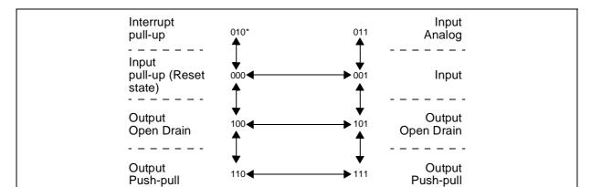
Figure 23. Diagram showing Safe I/O State Transitions
