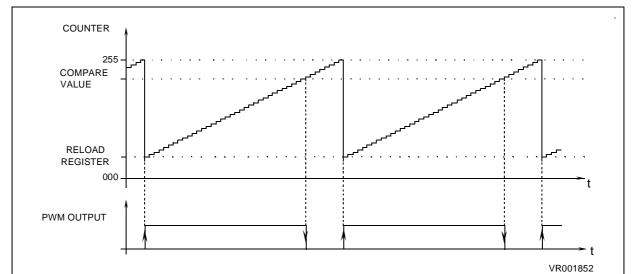
Figure 28. Auto-reload Timer PWM Function
