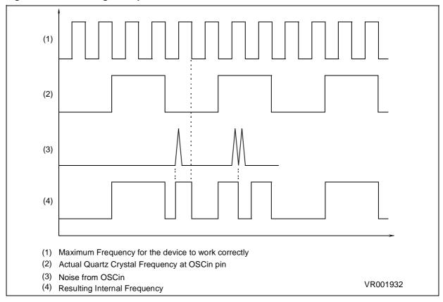
Figure 10. OSG Emergency Oscillator Principle
