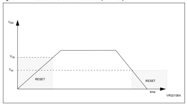
Figure 14. LVD Reset on Power-on and Power-down (Brown-out)
