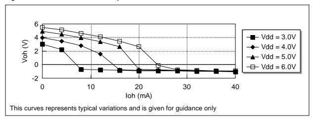
Figure 36. Voh versus Ioh on all I/O port at Vdd=5V
