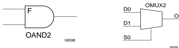
Figure 20: AND & MUX Symbols in XC4000X IOB
