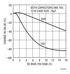
Figure 3. Ceramic Capacitor DC Bias Characteristics
