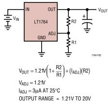
Figure 2. Adjustable Operation
