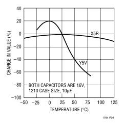
Figure 4. Ceramic Capacitor Temperature Characteristics
