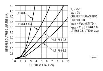
Figure 5. Reverse Output Current
