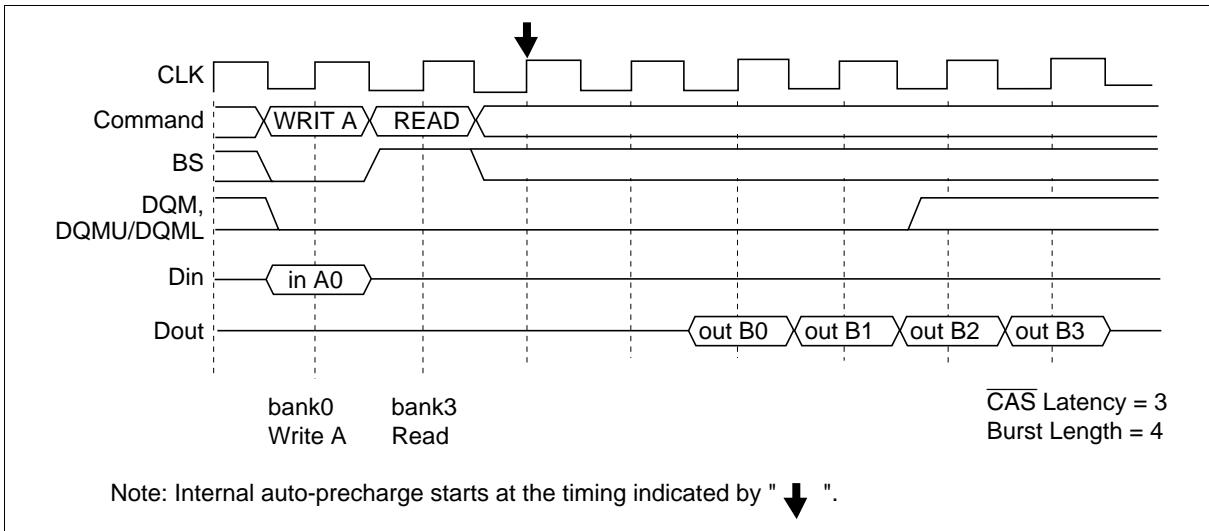
**Same bank:** The consecutive read command from write with auto precharge (the same bank) is illegal. It is necessary to separate the two commands with a bank active command.
