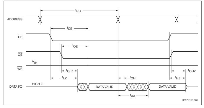
Notes: (4) t<sub>LZ</sub> min., t<sub>HZ</sub>, t<sub>OLZ</sub> min., and t<sub>OHZ</sub> are periodically sampled and not 100% tested. t<sub>HZ</sub> max. and t<sub>OHZ</sub> max. are measured from the point when CE or OE return HIGH (whichever occurs first) to the time when the outputs are no longer driven.
