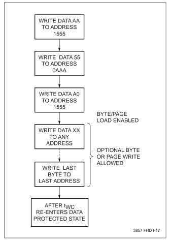
Regardless of whether the device has previously been protected or not, once the software data protection algorithm is used, the X28HC64 will automatically disable further writes unless another command is issued to deactivate it. If no further commands are issued the X28HC64 will be write protected during power-down and after any subsequent power-up.
