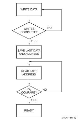
DATA Polling can effectively reduce the time for writing to the X28HC64. The timing diagram in Figure 2 illustrates the sequence of events on the bus. The software flow diagram in Figure 3 illustrates one method of implementing the routine.
