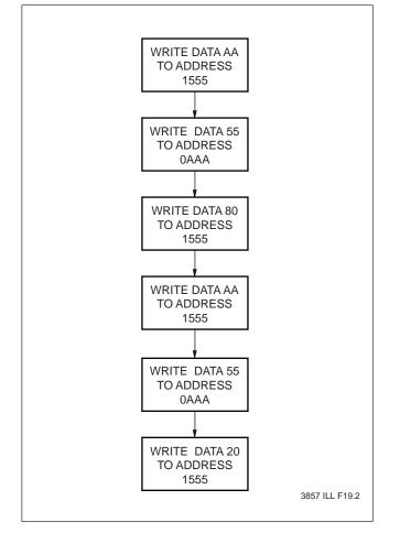
In the event the user wants to deactivate the software data protection feature for testing or reprogramming in an E<sup>2</sup>PROM programmer, the following six step algorithm will reset the internal protection circuit. After  $t_{WC}$ , the X28HC64 will be in standard operating mode.
