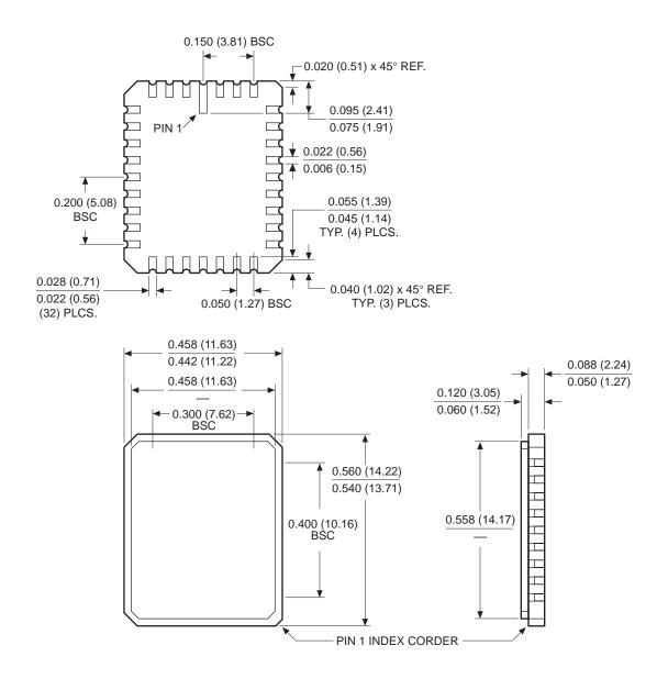
NOTE: 1. ALL DIMENSIONS IN INCHES (IN PARENTHESES IN MILLIMETERS) 2. TOLERANCE:  $\pm 1\%$  NLT  $\pm 0.005$  (0.127)
