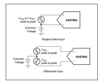
FIGURE 1. Methods of Driving the ADS7864 Single-Ended or Differential.
