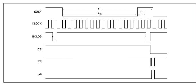
FIGURE 9. Timing of One Conversion Cycle.
