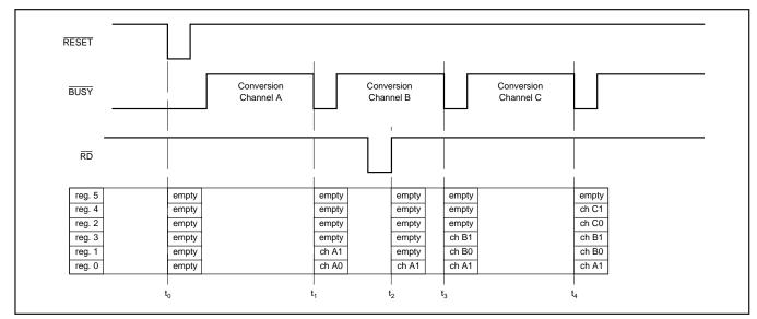
FIGURE 14. Functionality Diagram of FIFO Registers.
