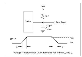
FIGURE 6. Test Circuits for Timing Specifications.
