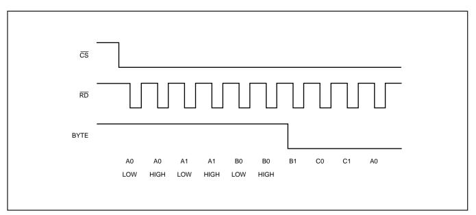
FIGURE 12. Reading Data in Cycling Mode.
