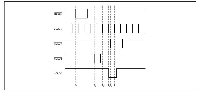
FIGURE 13. Example of Hold Signals.
