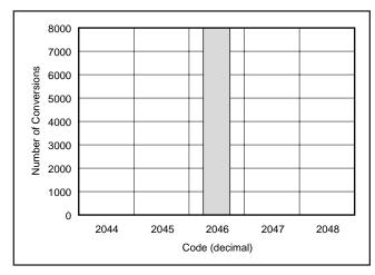
FIGURE 5. Histogram of 8,000 Conversions of a DC Input.
