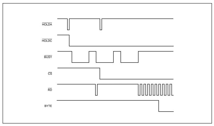
FIGURE 11. Reading Data in Cycling Mode.
