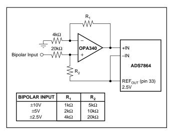
FIGURE 7. Level Shift Circuit for Bipolar Input Ranges.
