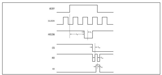
FIGURE 10. Timing for Reading Data.
