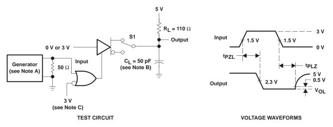
NOTES: A. The input pulse is supplied by a generator having the following characteristics: PRR  $\leq$  1 MHz, duty cycle = 50%, t<sub>r</sub>  $\leq$  5 ns, t<sub>f</sub>  $\leq$  5 ns, Z<sub>O</sub> = 50  $\Omega$ .
