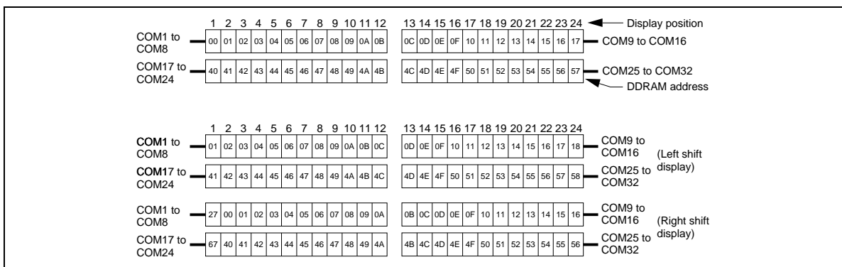
Figure 5 2-Line by 24-Character Display (5-Dot Font Width)
