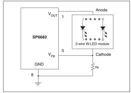
Figure 11. Driving 2-wire white LED module as current
