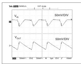
Figure 3. X2 mode voltage ripple when  $V_{IN} = 2.7V$
