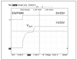
Figure 1. Output voltage turn-on time
