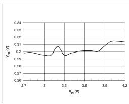
Figure 4. Feedback pin voltage vs. input voltage
