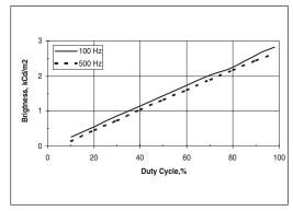
Figure 8. Brightness vs duty cycle
