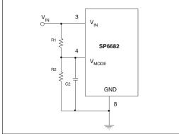
Figure 13. Programming the Vmode Resistors
