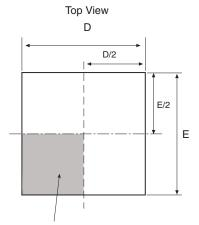
Pin 1 identifier to be located within this shaded area. Terminal #1 Index Area (D/2 \* E/2)
