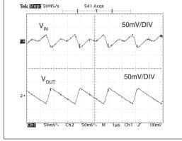
Figure 5. X1.5 mode voltage ripple when  $V_{IN} = 3.3V$
