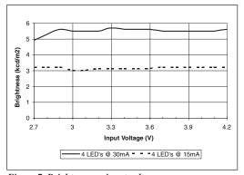
Figure 7. Brightness vs. input voltage
