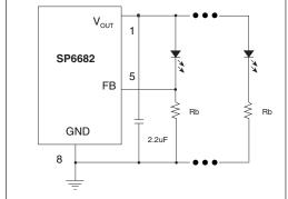
Figure 9. Driving discrete white LEDs as current source
