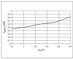
Figure 6. Quiescent current vs. input voltage
