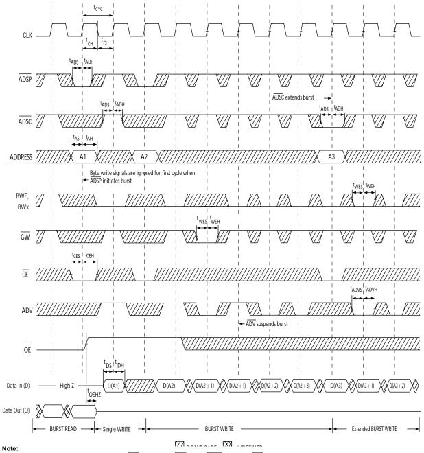
18. Full width write can be initiated by either  $\overline{GW}$  LOW; or by  $\overline{GW}$  HIGH,  $\overline{BWE}$  LOW and  $\overline{BW}_{[A:D]}$  LOW.
