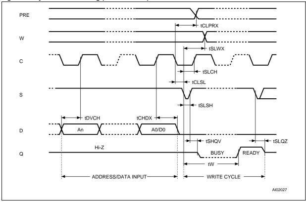
Figure 12. Synchronous Timing (Read or Write)
