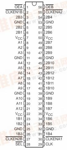
For data transfer in the A-to-B direction, a two-stage pipeline is provided in the A-to-1B path, with a single storage register in the A-to-2B path. Proper control of these inputs allows two sequential 12-bit words to be presented synchronously as a 24-bit word on the B port. Data flow is controlled by the active-low output enables (OEA, OEB). These control terminals are registered, so bus direction changes are synchronous with CLK.
