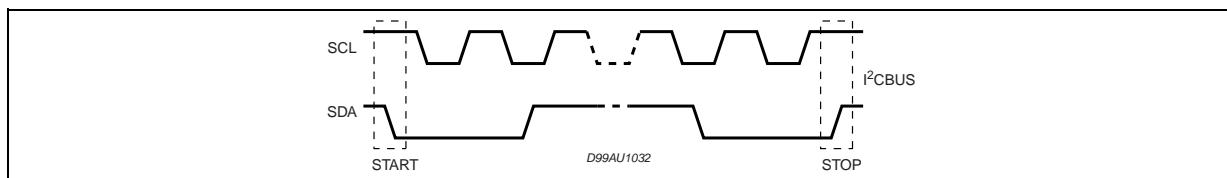
**Figure 8. Acknowledge on the I<sup>2</sup>CBUS**
