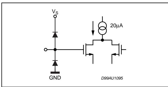
**Figure 15. PINS: BASSI\_L, BASSI\_R**
