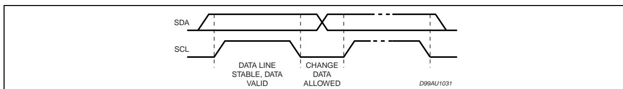
**Figure 7. Timing Diagram of I<sup>2</sup>CBUS**
