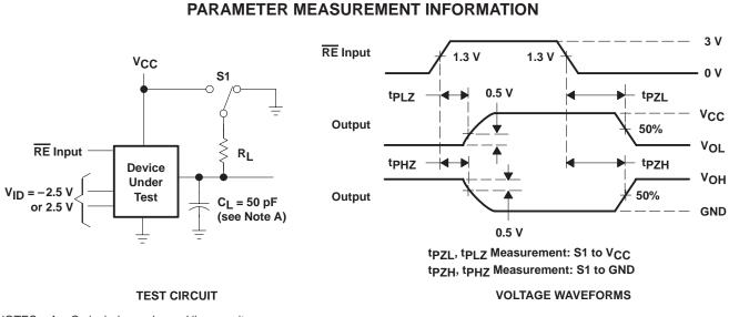
NOTES: A. CL includes probe and jig capacitance.
