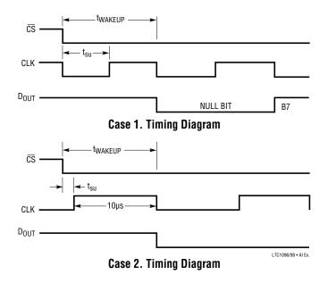
than 100kHz, Figure 1 shows the relationship between the wake-up time and setup time.
