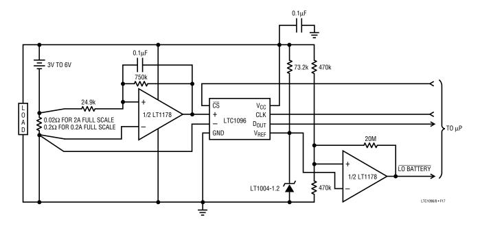
Figure 17. This OA to 2A Battery Current Monitor Draws Only 70µA from a 3V Battery
