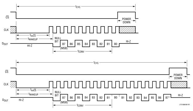
\*AFTER COMPLETING THE DATA TRANSFER, IF FURTHER CLOCKS ARE APPLIED WITH  $\overline{\text{CS}}$  LOW, THE ADC WILL OUTPUT ZEROS INDEFINITELY.
