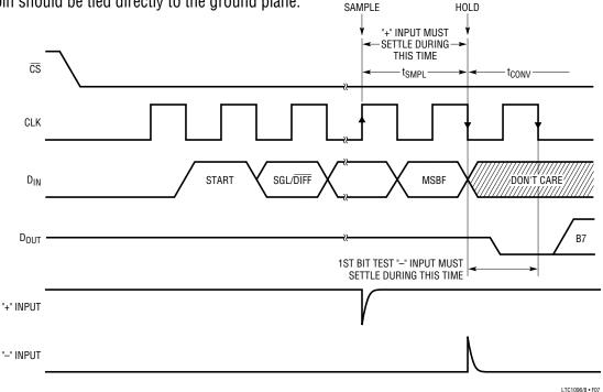
Figure 7. LTC1098(L) "+" and "-" Input Settling Windows
