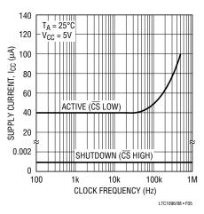
Figure 5. After a Conversion, When the Microprocessor Drives CS High, the ADC Automatically Shuts Down Until the Next Conversion. The Supply Current, Which Is Very Low During cConversions, Drops to Zero in Shutdown
