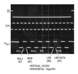
Figure 14. Scope Trace the LTC1096 "Quick Look" Circuit Showing A/D Output 10101010 (AA<sub>HFX</sub>)
