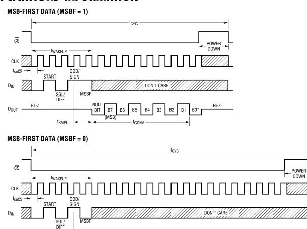
\*AFTER COMPLETING THE DATA TRANSFER, IF FURTHER CLOCKS ARE APPLIED WITH CS LOW, THE ADC WILL OUTPUT ZEROS INDEFINITELY.
