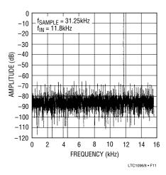
Figure 11. This Clean FFT of an 11.8kHz Input Shows Remarkable Performance for an ADC That Draws Only 100µA When Sampling at the 31.25kHz Rate
