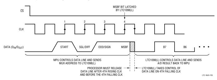
Figure 3. LTC1098(L) Operation with D<sub>IN</sub> and D<sub>OUT</sub> Tied Together
