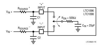
Figure 8. Analog Input Equivalent Circuit
