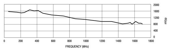
Figure 5. Output Amplitude versus Input Frequency
