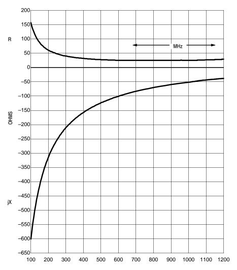
Figure 7. Typical Input Impedance versus Input Frequency
