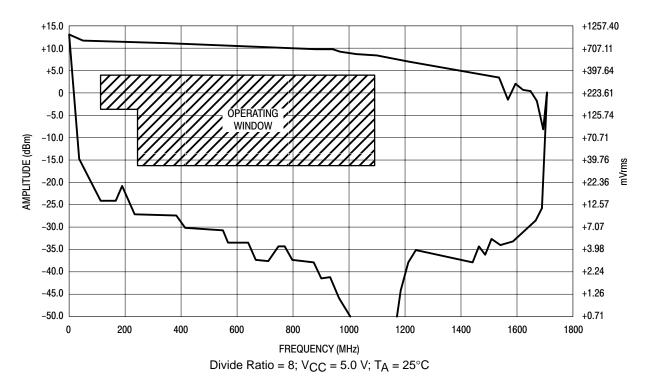
Figure 4. Input Signal Amplitude versus Input Frequency
