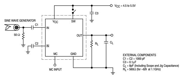
Figure 3. AC Test Circuit
