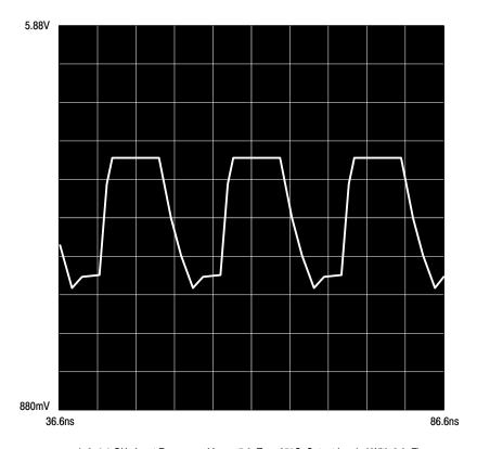
(÷8, 1.1 GHz Input Frequency,  $V_{CC}$  = 5.0,  $T_{A}$  = 25°C, Output Loaded With 8.0pF)
