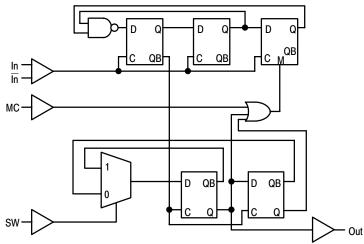
Figure 1. Logic Diagram (MC12026A)
