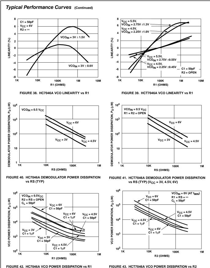
IRE 42. HG7046A VGO POWER DISSIPATION (C1 = 50pF,  $1\mu$ F)
