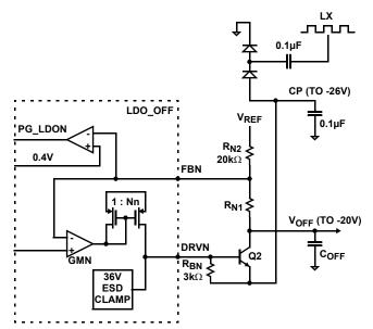
FIGURE 29. VOFF FUNCTIONAL BLOCK DIAGRAM
