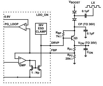
FIGURE 28. VON FUNCTIONAL BLOCK DIAGRAM
