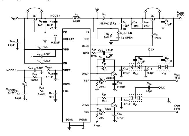
NOTE: The SGND should be connected to the exposed die plate and connected to the PGND at one point only.
