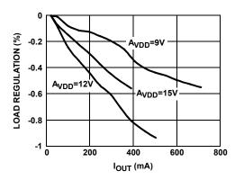
FIGURE 6.  $V_{BOOST}$  LOAD REGULATION AT  $V_{IN}$  = 5V (PI MODE)
