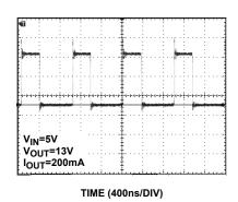
FIGURE 22. LX WAVEFORM - CONTINUOUS MODE
