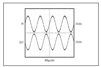
Figure 3. Rail-to-Rail Input/Output Voltage Range
