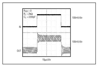
Figure 6b. Pulse Response Without Isolating Resistor
