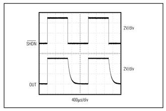
Figure 5. Shutdown Waveform
