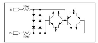
Figure 2. Input Protection Circuit
