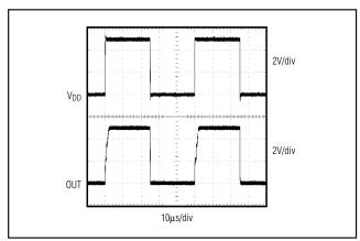
Figure 4. Power-Up/Power-Down Waveform
