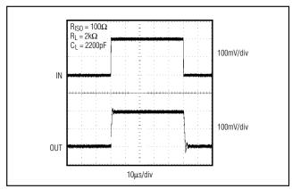
Figure 6c. Pulse Response With Isolating Resistor
