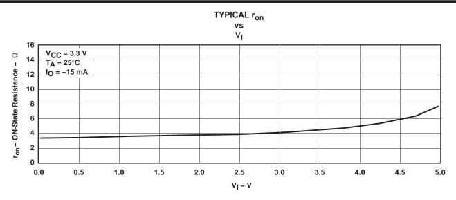
Figure 1. Typical  $r_{on}$  vs  $V_{I}$ ,  $V_{CC}$  = 3.3 V and  $I_{O}$  = -15 mA
