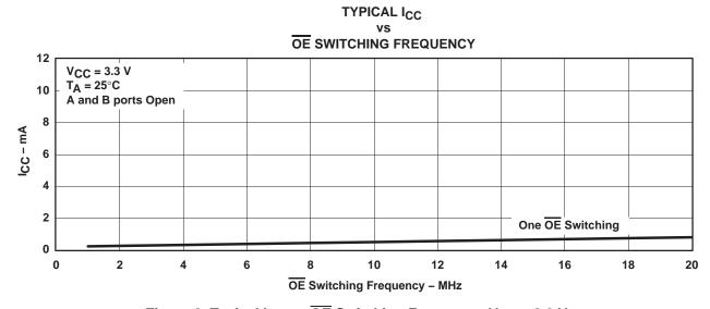
Figure 2. Typical I<sub>CC</sub> vs  $\overline{\text{OE}}$  Switching Frequency, V<sub>CC</sub> = 3.3 V
