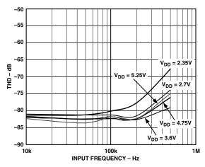
Figure 9. THD vs. Analog Input Frequency,  $f_S = 993 \text{ kSPS}$
