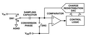
Figure 3. ADC Conversion Phase
