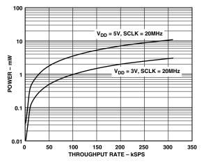
Figure 14. Power vs. Throughput Rate
