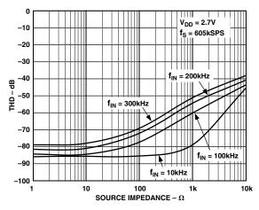
Figure 8. THD vs. Source Impedance for Various Analog Input Frequencies
