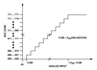
Figure 5. Transfer Characteristic for AD7478
