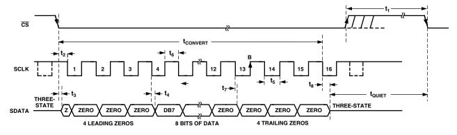
Figure 17. AD7478 Serial Interface Timing Diagram
