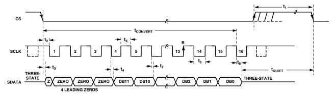
Figure 15. AD7476 Serial Interface Timing Diagram
