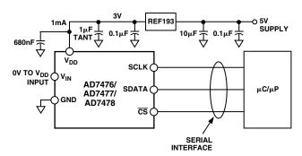
Figure 6. REF193 as Power Supply to AD7476/AD7477/ AD7478
