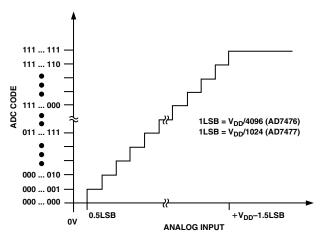
Figure 4. Transfer Characteristic for the AD7476/AD7477
