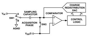
Figure 2. ADC Acquisition Phase
