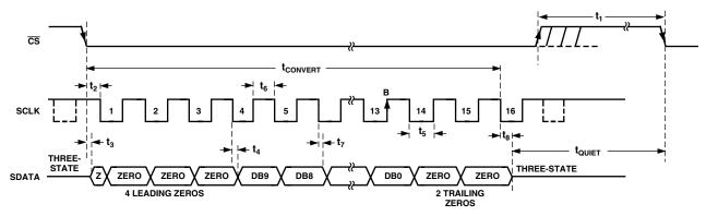
Figure 16. AD7477 Serial Interface Timing Diagram
