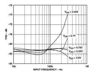
Figure 10. THD vs. Analog Input Frequency,  $f_S = 605 \text{ kSPS}$
