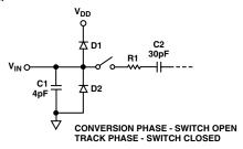
Figure 7. Equivalent Analog Input Circuit
