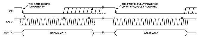
Figure 13. Exiting Power-Down Mode
