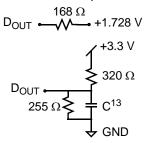
Figure B: 3.3 V Output load
