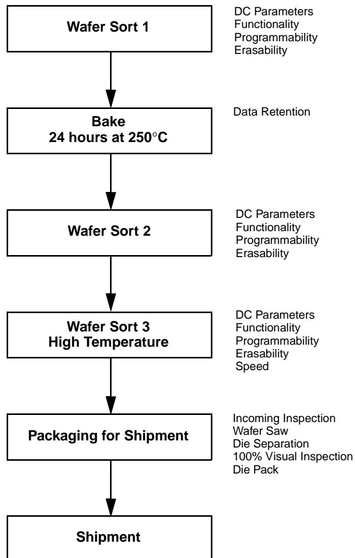
Figure 1. AMD KGD Product Test Flow
