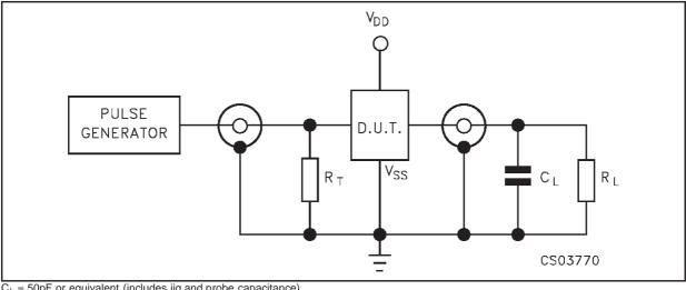
$C_L = 50 \text{pF}$  or equivalent (includes jig and probe capacitance)  $R_L = 200 K \Omega$   $R_T = Z_{OUT}$  of pulse generator (typically 50  $\Omega$ )
