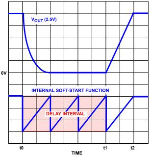
FIGURE 5. OVERCURRENT PROTECTION RESPONSE
