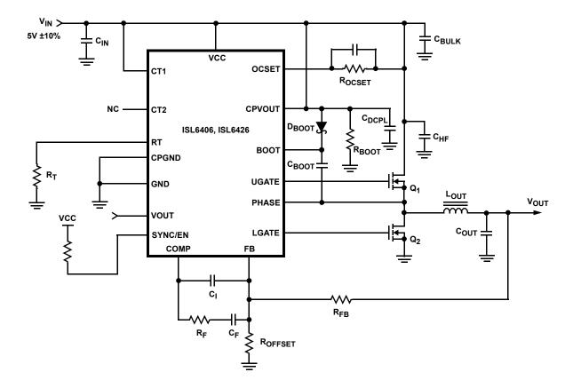
Typical Application Schematic for 5V Input
