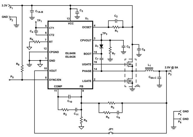
NOTE: Remove R3, R4, C9, and R5 from the board and close JP1 for ISL6426 evaluation.
