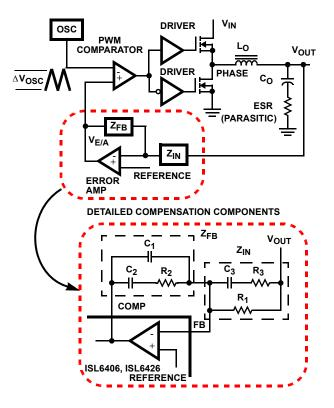
FIGURE 7. VOLTAGE-MODE BUCK CONVERTER COMPENSATION DESIGN
