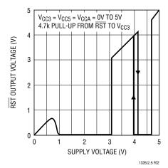
Figure 2. RST Voltage vs Supply Voltage
