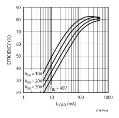
Figure 4b. P<sub>OUT</sub>/P<sub>IN</sub> Efficiency
