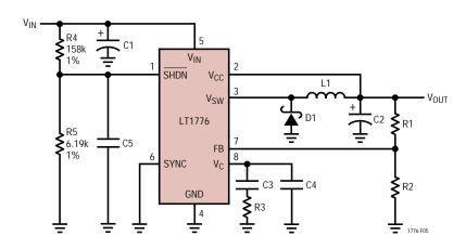
Figure 5. User Programmable Undervoltage Lockout
