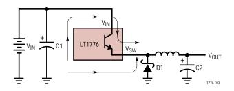
Figure 3. High Speed Current Switching Paths
