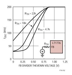
Figure 2. Oscillator Frequency vs FB Divider Thevenin Voltage and Impedance
