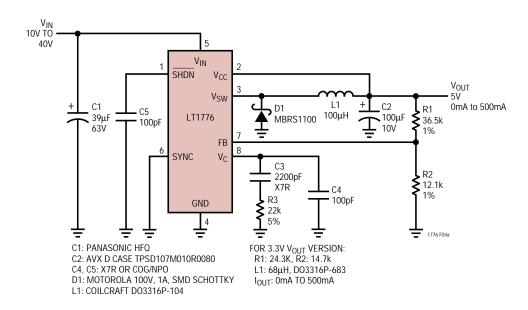
Figure 4a. Minimum Component Count Application
