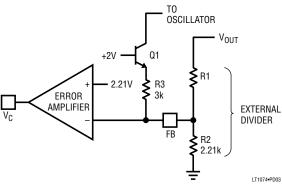
Figure 3. Frequency Shifting
