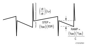
Figure 1. Input Capacitor Ripple
