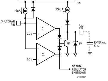
Figure 5. Shutdown Circuitry
