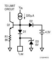
Figure 8. ILIM Pin Circuit
