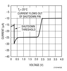
Figure 4. Shutdown Pin Characteristics
