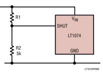
Figure 6. Undervoltage Lockout
