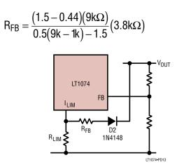
Figure 9. Foldback Current Limit
