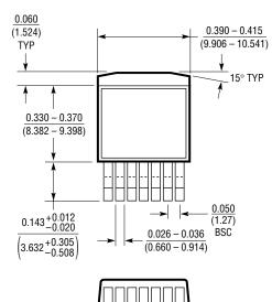
R Package 7-Lead Plastic DD Pak (LTC DWG # 05-08-1462)
