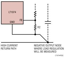
Figure 2. Proper Ground Pin Connection
