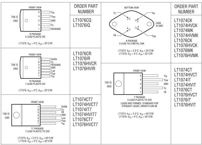
\*Assumes package is soldered to 0.5 IN<sup>2</sup> of 1 oz. copper over internal ground plane or over back side plane.
