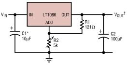
\*NEEDED IF DEVICE IS FAR FROM FILTER CAPACITORS
