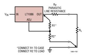
Figure 2. Connections for Best Load Regulation
