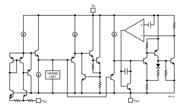
The LT1086 family of 3-terminal regulators is easy to use and has all the protection features that are expected in high performance voltage regulators. They are short-circuit protected, have safe area protection as well as thermal shutdown to turn off the regulator should the temperature exceed about 165°C at the sense point.
