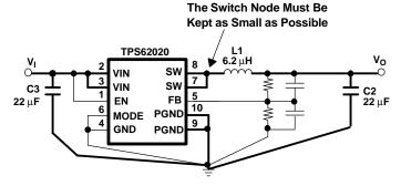
Figure 16. Layout Diagram
