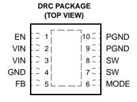
NOTE: The PowerPAD must be connected to GND.
