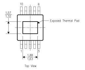
NOTE: All linear dimensions are in millimeters
