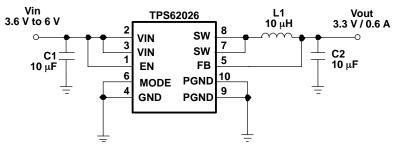
Figure 21. TPS62026 Fixed 3.3 V Output Using 10 µH inductor
