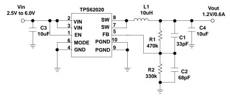
Figure 19. 1.2 V Output Using 10 µH Inductor
