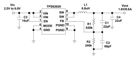
Figure 18. 1.8 V Output Using 6.8 µH Inductor
