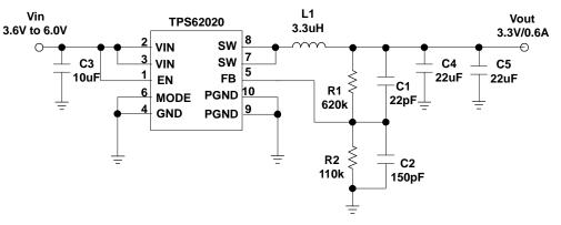
Figure 17. Li-Ion to 3.3 V With Improved Load Transient Response
