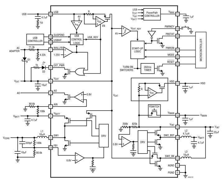
Figure 1. LTC3456 Block Diagram
