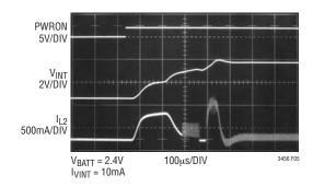
Figure 5. Inrush Current at Power-Up (Battery Powered)
