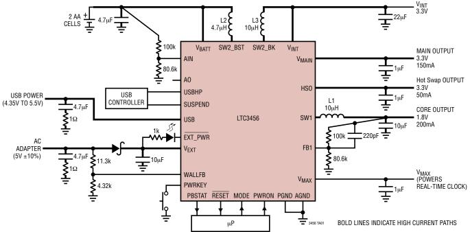
Figure 16. Layout Diagram
