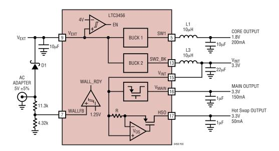
Figure 3. AC Adapter-Powered LTC3456
