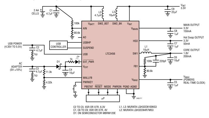
Figure 17. 2 AA Cells to 1.8V/200mA and 3.3V/200mA Outputs Using All Ceramic Capacitors with Lowest Parts Count
