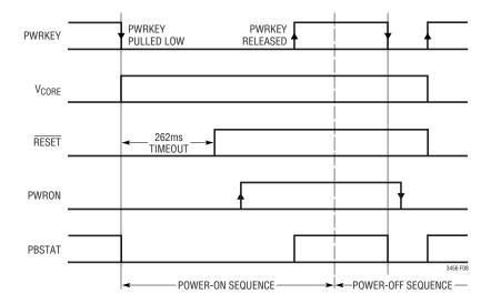
Figure 8. Power-On/Power-Off Sequence
