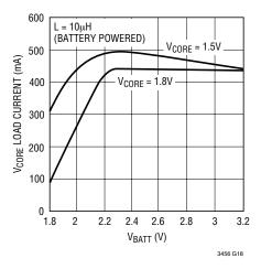
Figure 7. Maximum Output Current vs Battery Voltage
