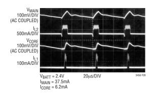
Figure 9. The LTC3456 in Burst Mode Operation
