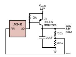
Figure 11. Generating Auxiliary Voltage Supply
