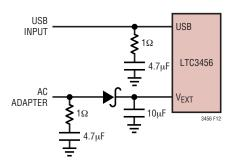
Figure 12. Bypassing USB and AC Wall Adapter Inputs
