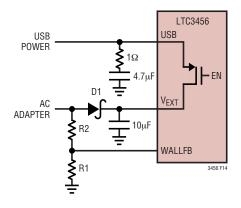
Figure 14. Setting the Wall Adapter UVLO Voltage
