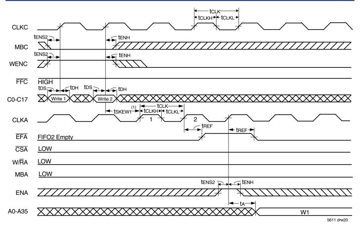
Figure 19. EFA Flag Timing and First Data Read when FIFO2 is Empty (IDT Standard Mode)
