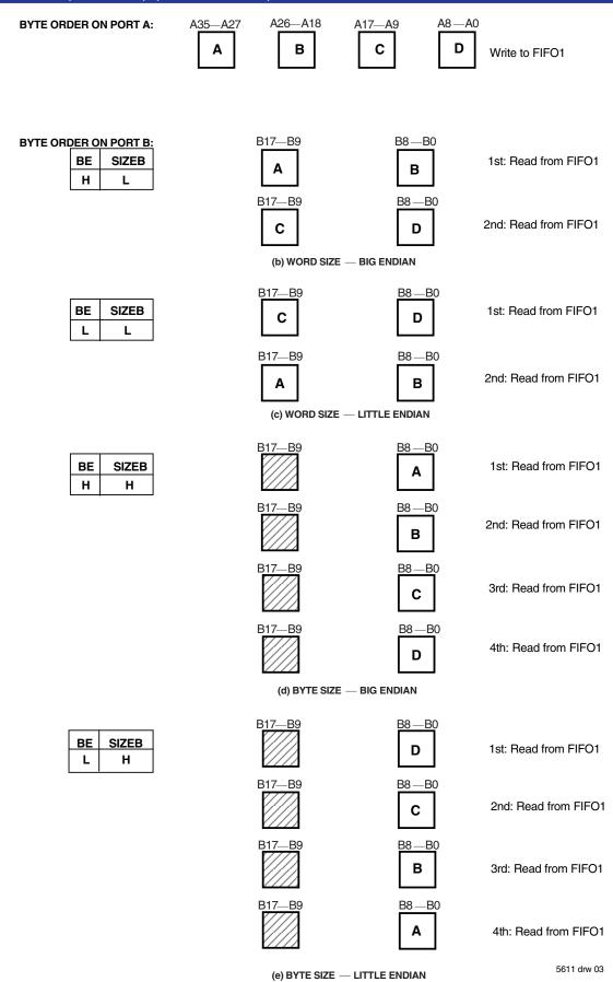
Figure 2. Port B Bus Sizing
