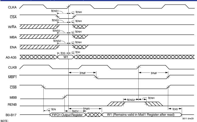
1. If Port B is configured for word size, data can be written to the Mail1 register using A0-A17 (A18-A35 are don't care inputs). In this first case B0-B17 will have valid data. If Port B is configured for byte size, data can be written to the Mail1 Register using A0-A8 (A9-A35 are don't care inputs). In this second case, B0-B8 will have valid data (B9-B17 will be indeterminate).
