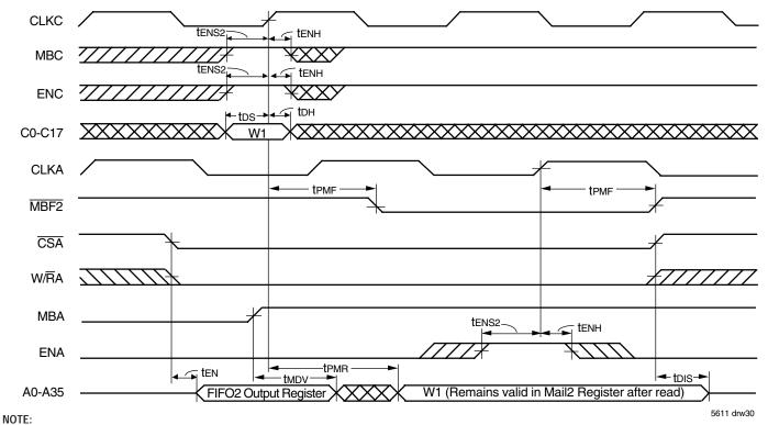
1. If Port C is configured for word size, data can be written to the Mail2 register using C0-C17. In this first case, A18-A35 will have valid data (A0-A17 will be indeterminate). If Port C is configured for byte size, data can be written to the Mail2 register using C0-C8 (C9-C17 are don't care inputs). In this second case, A18-A26 will have valid data (A0-A17 and A27-A35 will be indeterminate).
