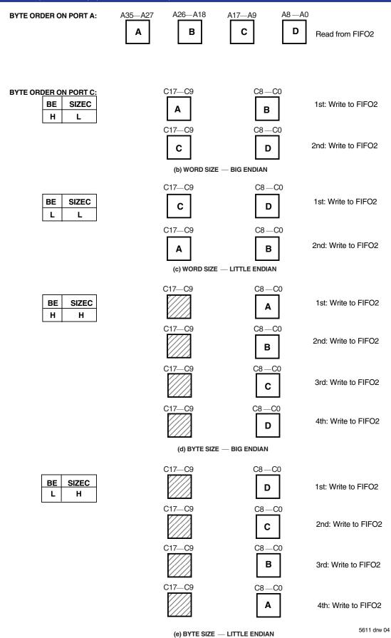
Figure 3. Port C Bus Sizing
