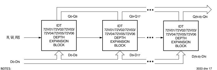
For depth expansion block see section on Depth Expansion and Figure 14.
