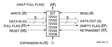
Figure 12. Block Diagram of Single 512 x 9, 1,024 x 9, 2,048 x 9, 4,096 x 9, 8,192 x 9 and 16,384 x 9 FIFO
