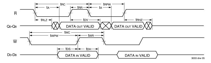
Figure 3. Asynchronous Write and Read Operation
