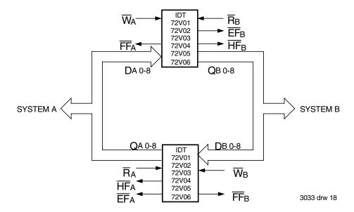
Figure 16. Bidirectional FIFO Mode
