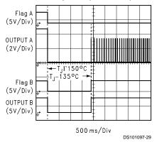
\* Port A is shorted to GND through a 100 m $\Omega$  resistor
