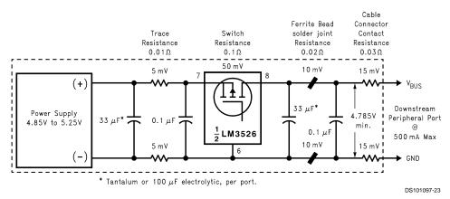
FIGURE 2. Self-Powered Hub Per-Port Voltage Drop
