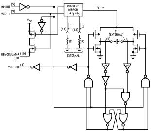
FIGURE 2. Logic Diagram for VCO
