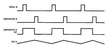
FIGURE 9. Typical Waveforms for Phase Comparator III
