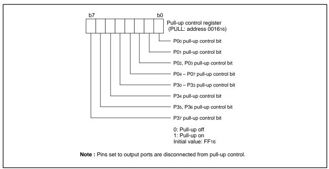
Fig. 9 Structure of pull-up control register
