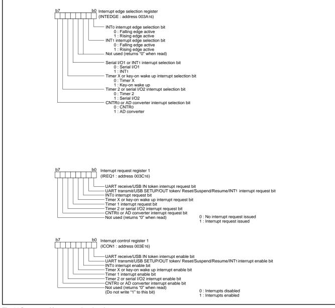
Fig. 14 Structure of interrupt-related registers
