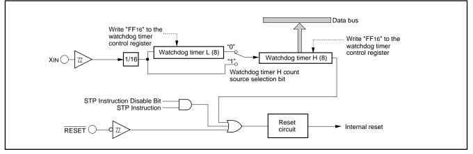
Fig. 35 Block diagram of watchdog timer
