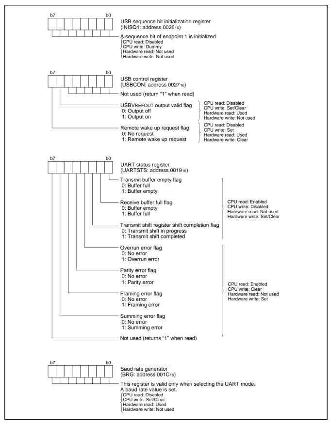
Fig. 27 Structure of serial I/O1-related registers (4)
