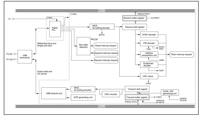
Fig. 22 USB mode block diagram
