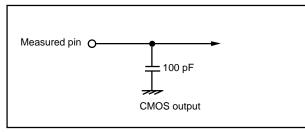
Fig. 46 Switching characteristics measurement circuit
