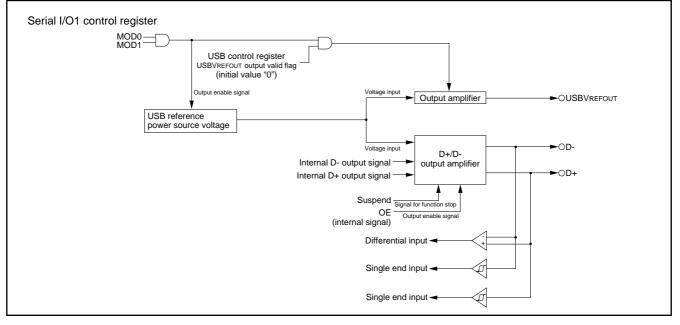
Fig. 23 USB transceiver block diagram
