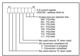
Fig. 32 Structure of A-D control register
