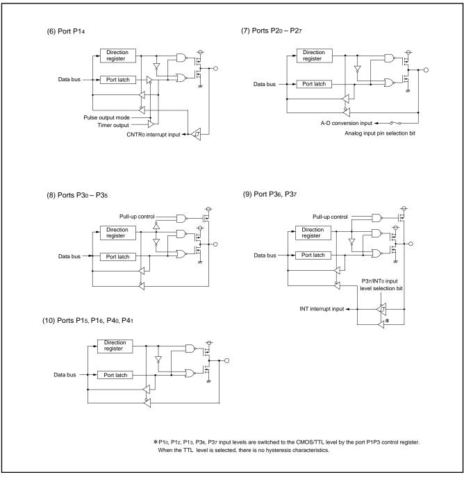
Fig. 12 Block diagram of ports (2)
