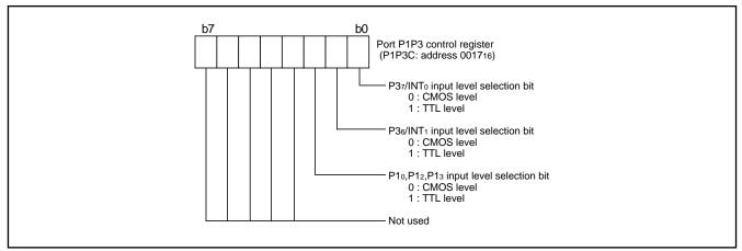
Fig. 10 Structure of port P1P3 control register
