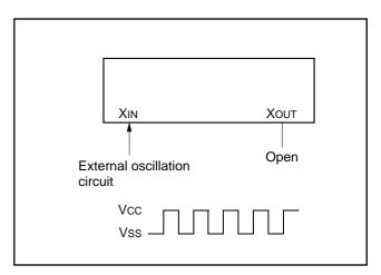
Fig. 41 External clock input circuit
