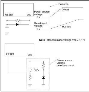
Fig. 37 Example of reset circuit
