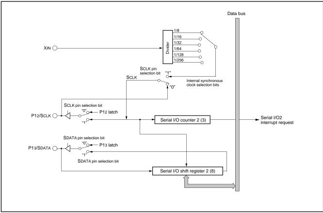
Fig. 30 Block diagram of serial I/O2
