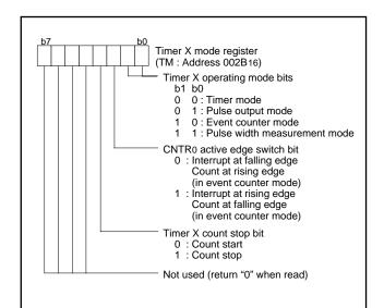
Fig. 16 Structure of timer X mode register
