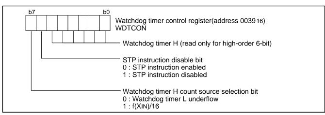
Fig. 36 Structure of watchdog timer control register
