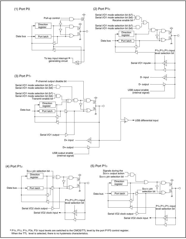
Fig. 11 Block diagram of ports (1)
