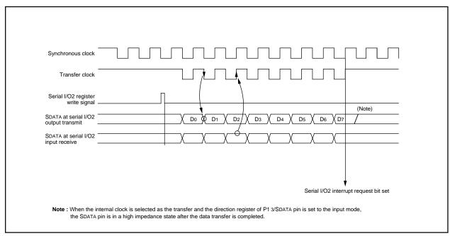
Fig. 31 Serial I/O2 timing (LSB first)
