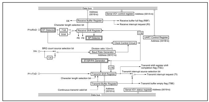
Fig. 19 Block diagram of UART serial I/O
