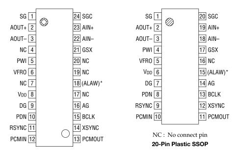
NC: No connect pin **24-Pin Plastic SOP**
