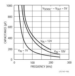
Figure 3. Timing Capacitor Value
