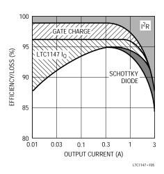
Figure 5. Efficiency Loss
