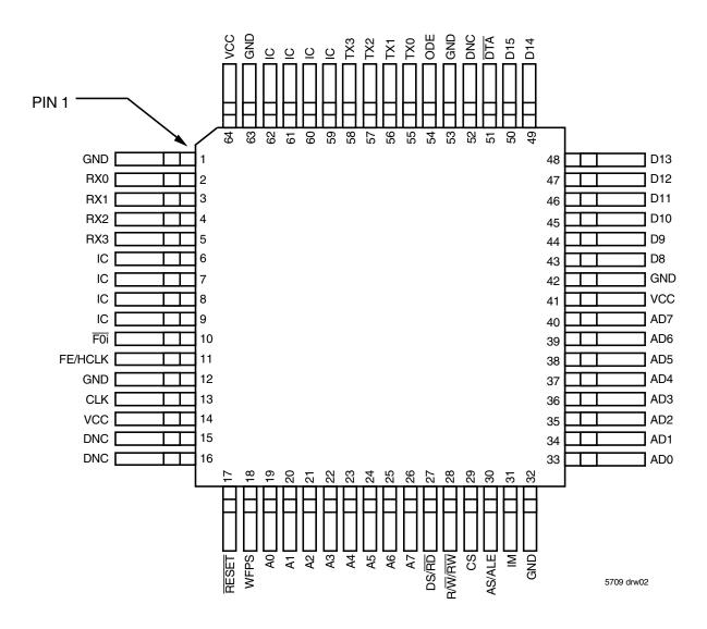
TQFP: 0.80 pitch, 14mm x 14mm (PN64-1, order code: PF) STQFP: 0.50 pitch, 10mm x 10mm (PP64-1, order code: TF) TOP VIEW
