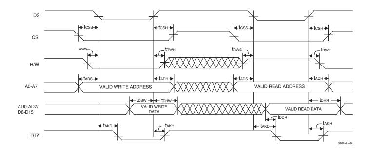
Figure 14. Motorola Non-Multiplexed Asyncronous Bus Timing
