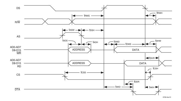
Figure 13. Multiplexed Bus Timing (Motorola Mode)
