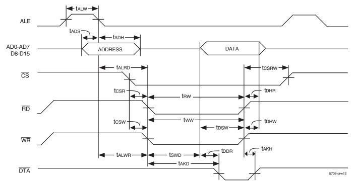
Figure 12. Multiplexed Bus Timing (Intel Mode)
