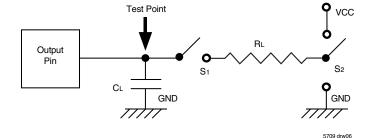
Figure 6. Output Load
