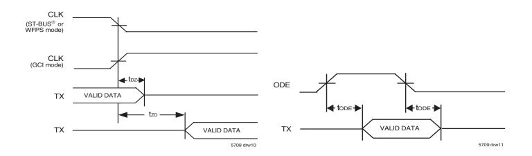
Figure 10. Serial Output
