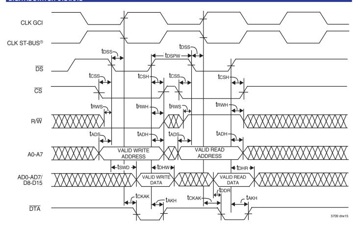
Figure 15. Motorola Non-Multiplexed Syncronous Bus Timing
