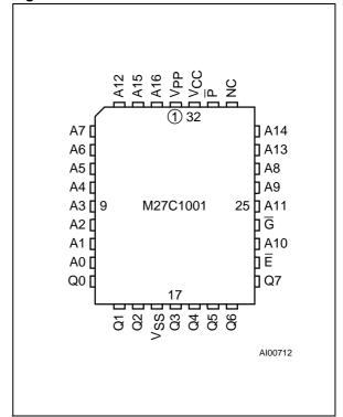
Figure 2C. TSOP Connections
