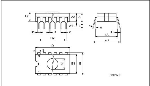
Table 14. PDIP32 - 32 lead Plastic DIP, 600 mils width, Package Mechanical Data
