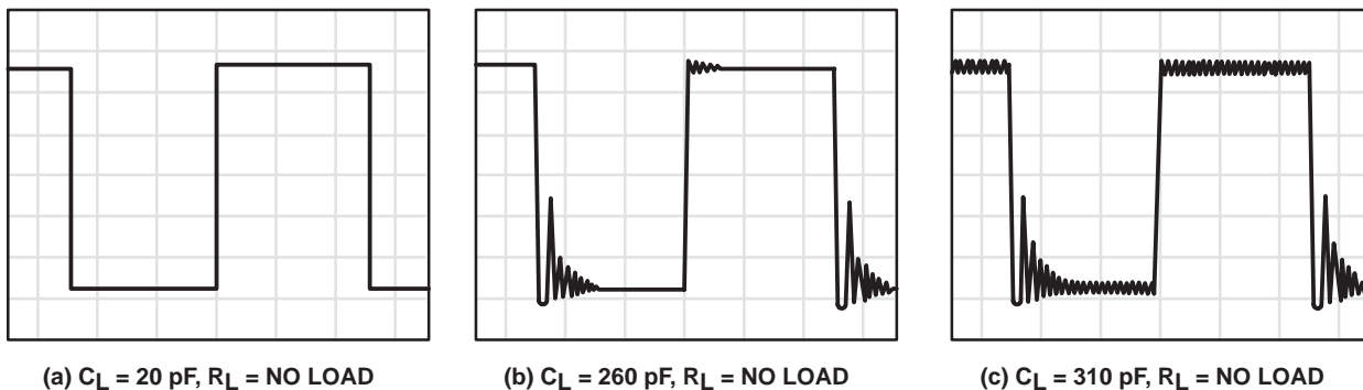
Figure 112. Effect of Capacitive Loads in Low-Bias Mode
