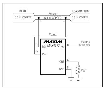
Figure 2. MAX4172 Connections Showing Use of PC Board
