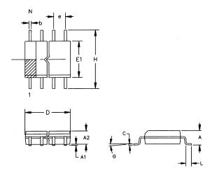
The chamfer on the body is optional. If it is not present, a terminal 1 identifier must be positioned so that 1/2 or more of its area is contained in the hatched zone.
