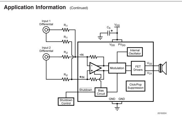
FIGURE 4. Dual Differential Input Configuration
