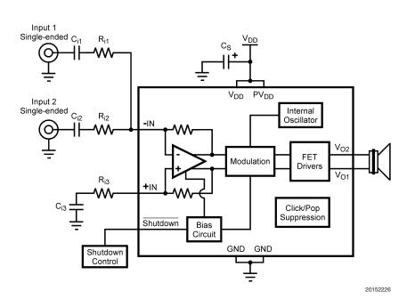
FIGURE 6. Dual Single-Ended Input Configuration
