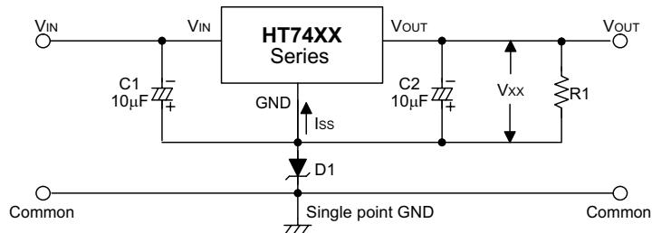
$$V_{OUT} = V_{xx} + V_{D1}$$
