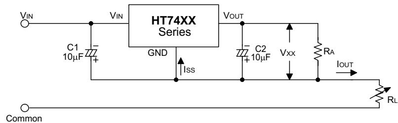
$$I_{OUT} = \frac{V_{xx}}{R_A} + I_{ss}$$
