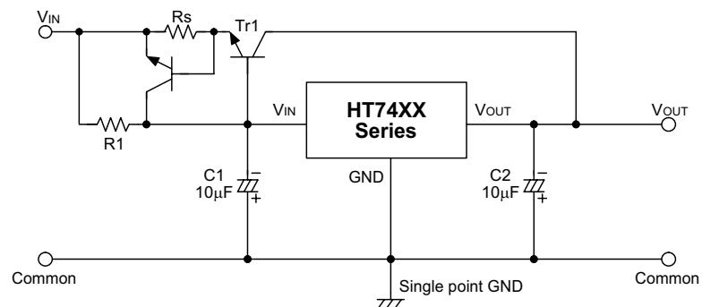
**Circuit for increasing output voltage**
