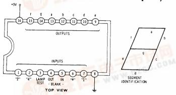
This package accepts a 1-2-4-8 positive-logic Binary Coded Decimal input and converts it to the proper pattern to light a 7-segment display. A low output is intended to light the segment.
