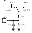
\*Includes jig and probe capacitance.
