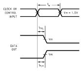
FIGURE 5. Propagation Delay, Pulse Width Waveforms
