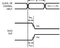
FIGURE 6. Propagation Delay, Pulse Width Waveforms
